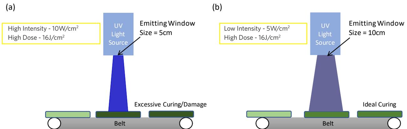
**Figure 5. (a)** In this instance the intensity and dose are too high resulting in damage to the target substrate producing an “overcure”. **(b)** In this instance, the intensity and dose level has been optimized to produce an ideal cure.
