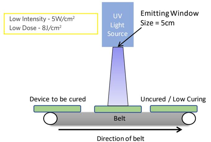
**Figure 4.** The image shows a UV LED lamp utilized for curing a device on a production line. At the stated intensity and dose, the device on the production line remains uncured or has only cured partially. In this case, the intensity and dose are both too low.
