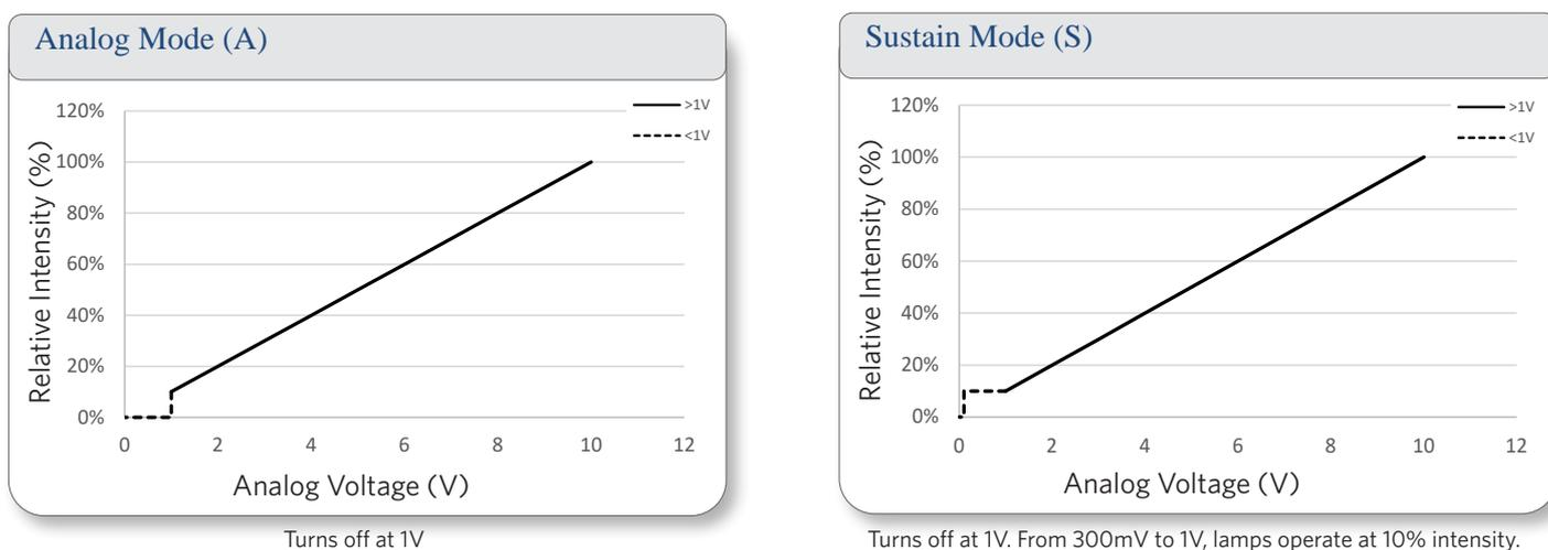
**Figure 7.** The first graph shows ProPhotonix “Analog mode” where intensity response turns on at 1V and linearly scales to 100% intensity at 10V. The second graph shows ProPhotonix’ “Sustain mode” turns on at 300mV. From 300mV to 1V the lamp operates at 10% intensity. From 1V, the lamp linearly scales to 100% intensity to 10V.
