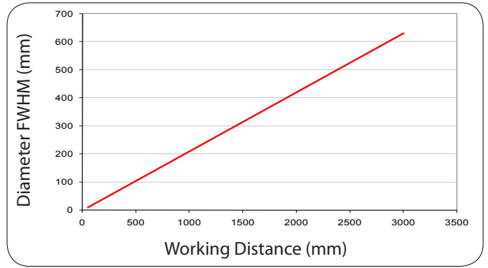
Figure 2 - Diameter of field of illumination vs. working distance for all wavelengths. For other wavelengths use ratio or irradiance of desired colour to red from Illumination Characteristics table on previous page
